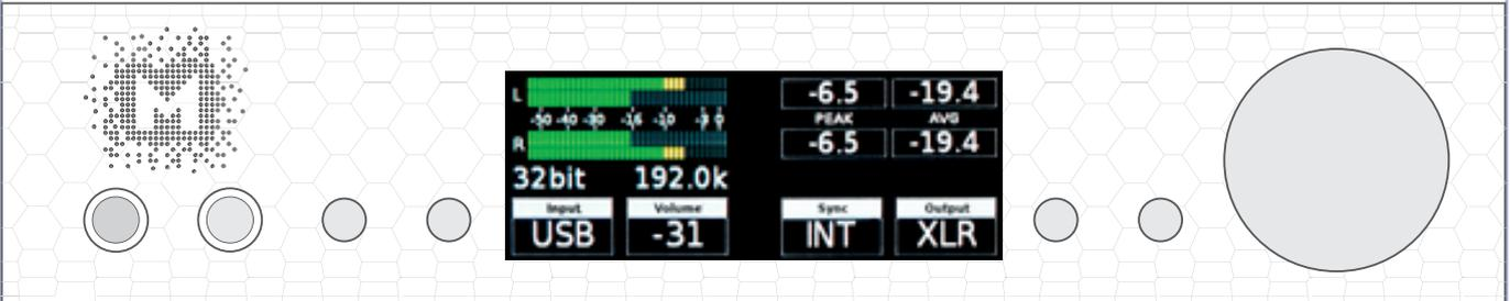
To enter the one of four parameters menu shown on the display, press one of the four buttons located on the left and right side of LCD display. When the value is ready to change it is back-lit with blue colour. To change the value rotate the knob until you see the option / value you need. Press the knob (or the same button) again to leave the menu.
