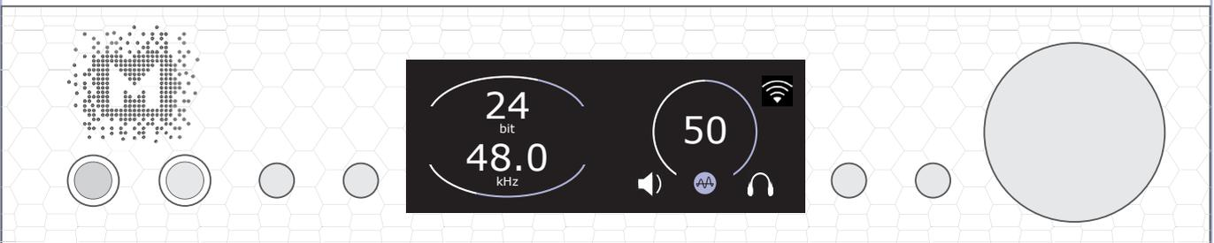
Press and hold the knob to switch the Brooklyn Bridge off / on.
